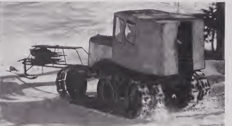
FIGURE 8. The Utah snowmobile, one variety of conventional Caterpillar tractor modified for use in snow, with forward skis for steering.
